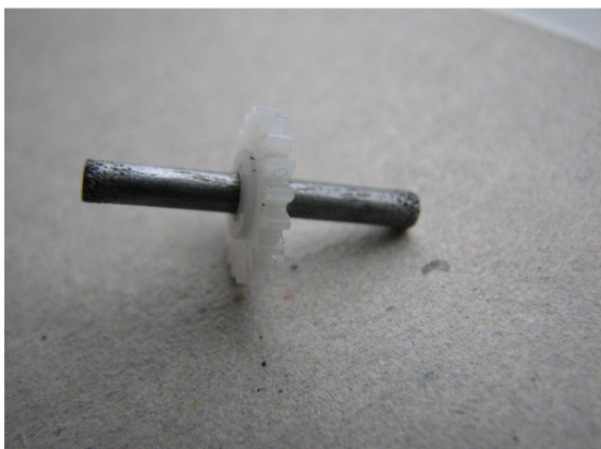
Gear pressed onto the centre of the axle.
