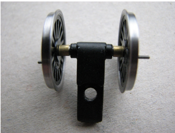
Leading wheel set assembled.
